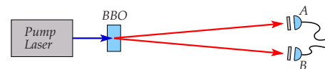
Fig. 2. A pump laser undergoes spontaneous parametric down conversion in a \beta -barium borate (BBO) crystal. The down-converted light is filtered before hitting the couplers. Although most of the pump laser passes unaffected through the crystal, we omit this beam from the diagram for clarity.
