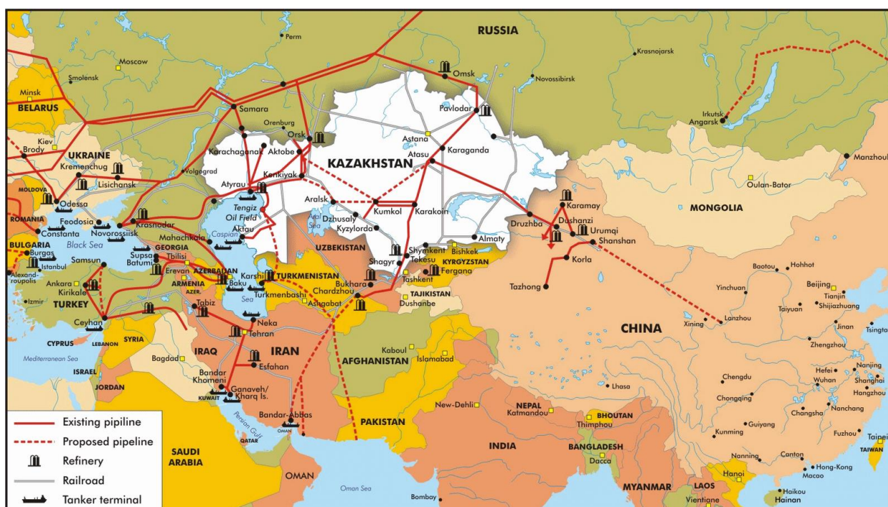
Fig. 2: Map showing oil pipelines (solid red lines) in Central Asia. Most pipelines go to Russia. The Baku-Tbilisi-Ceyhan route crosses the Caspian Sea from Aktau, the site of the Tengiz oil field, in western Kazakhstan. Oil enters China at Druzhba on Kazakhstan's eastern border. The other non-Russian pipeline reaches Turkmenistan via Uzbekistan (Energy Information Administration, 2012).
