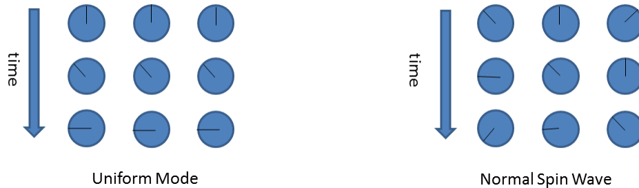
Figure 2.3: Uniform mode, and an example of a different spin wave. This diagram shows the planar component of the magnetic moment at a certain time t . For the uniform mode, the spins always remain in phase as time progresses. Other spin waves have a phase offset between different lattice points which persists as time progresses.
